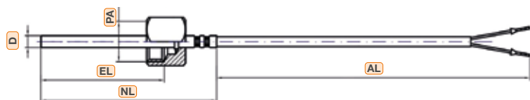
4: Stepped protection tube and loose internal thread
