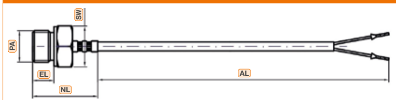
1: Cable temperature probe with thread and hexagon
