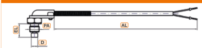
3: Bent protection tube and loose threaded connection with spring
