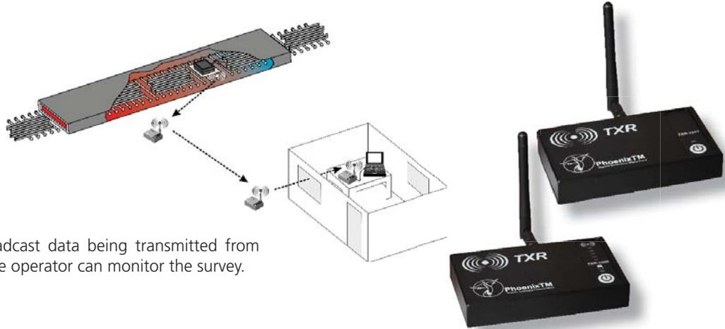
A series of routers can pick up and re-broadcast data being transmitted from within a furnace, to a remote office where the operator can monitor the survey.
