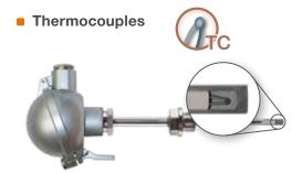
Temperature sensors may optionally be equipped with thermocouples type R, S, B, J, T, E, K, N, C and A according to DIN EN 60584, and can also be realised as versions with two or more thermocouples.
